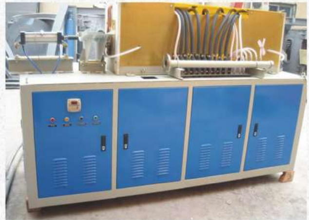
Induction heating cabinet-2
